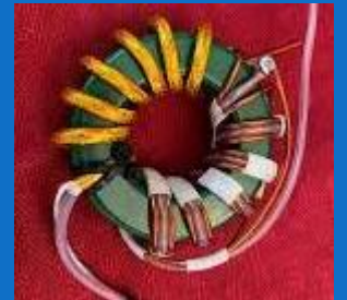
Balun for the DE which can arc when it get wet
