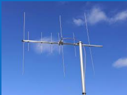
A UHF Yagi inside a VHF Yagi
