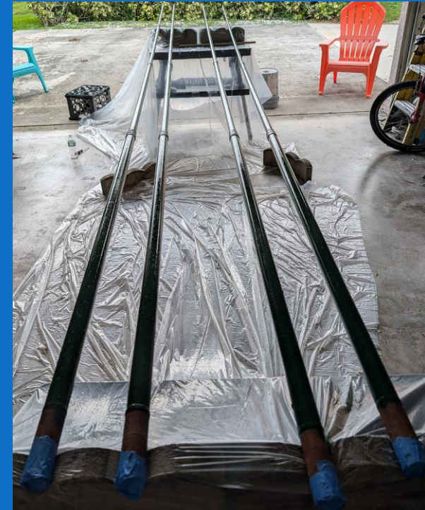
The fiberglass tubes were stored with the open ends covered with painters tape to keep bugs and lizards from getting inside
